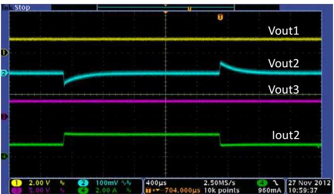
Figure 23. Transient Response Buck2@1.8V, 1-2A Step, C_o = 47\mu\text{F}
